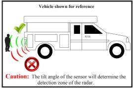
The PreView\* system is a blind spot collision warning system designed to supplement other safety practices and/or devices. The machine operator is always the first line of defense when safely operating a vehicle.
