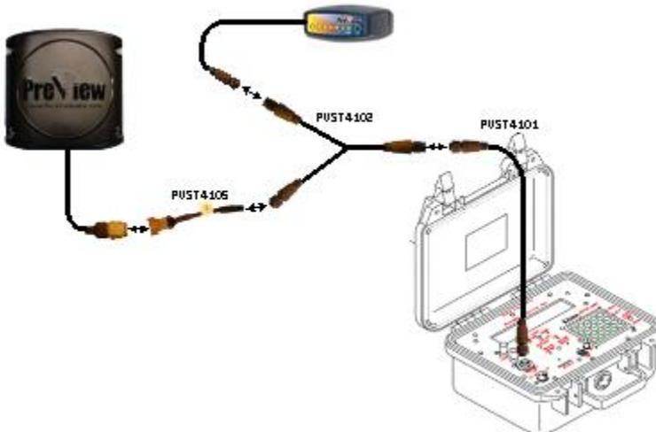
Cable PVST4102 is used for network diagnostics and troubleshooting. It cannot be used to configure a sensor or display unless **all** devices support the PrecoNet 2.0 protocol. This cable is designed to interface with an installed system. Since the Service Tool can only power 1 device at a time, this cable allows the machine to power the entire system while enabling Service Tool communication.
