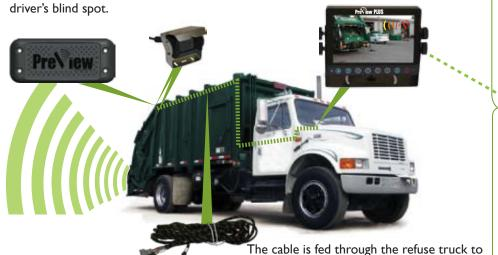
connect the sensors to the in-cab monitor.
