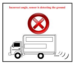
The Sensor should be centered on the rear of the vehicle for best coverage. **Caution:** The tilt angle of the sensor will determine the path of the radar. (See images above)
