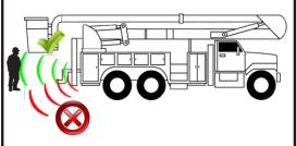
**Caution:** The tilt angle of the sensors will determine the detection zone of the radar.
