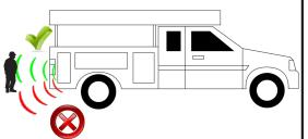
**Caution:** The tilt angle of the sensor will determine the detection zone of the radar.
