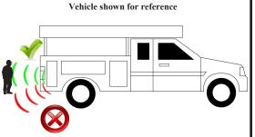
**Caution:** The tilt angle of the sensor will determine the detection zone of the radar.
