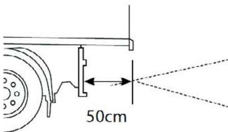
50cm compensation range for sensors fitted inboard of vehicle rear (selectable via dip switch)
