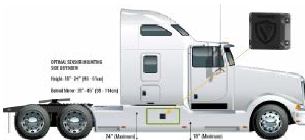
Figure 6. Sensor Position on Vehicle
