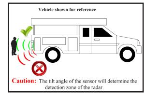
The PreView<sup>®</sup> system is a blind spot collision warning system designed to supplement other safety practices and/or devices. The machine operator is always the first line of defense when safely operating a vehicle.
