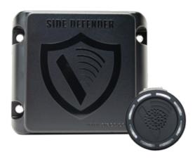
One such example is the PreView Side Defender®II. By adding new technology to PRECO's already successful lane change assist feature, the new system alerts operators on moving vulnerable road users (VRU) in crowded urban environments.
