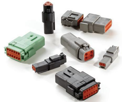
DEUTSCH DTM series connectors offer solutions to your smaller wire gauge applications. Building on the DT design strengths, the DTM connector line was developed to fill the need for lower amperage, multi-pin connectors. The DTM series offers the designer the ability to use multiple size 20 contacts, each with 7.5 amp continuous capacity, within a single shell.
