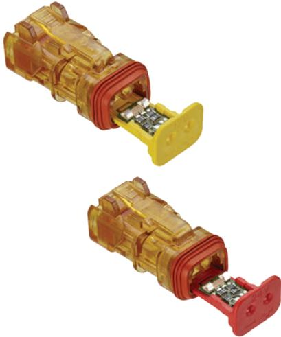
The Detector connector has an integrated LED used for diagnostics. The transparent housing features reduced diameter seals and may be ordered with or without an end cap. Color coded wedgelocks for operating voltages, 12VDC and 24VDC are available.
