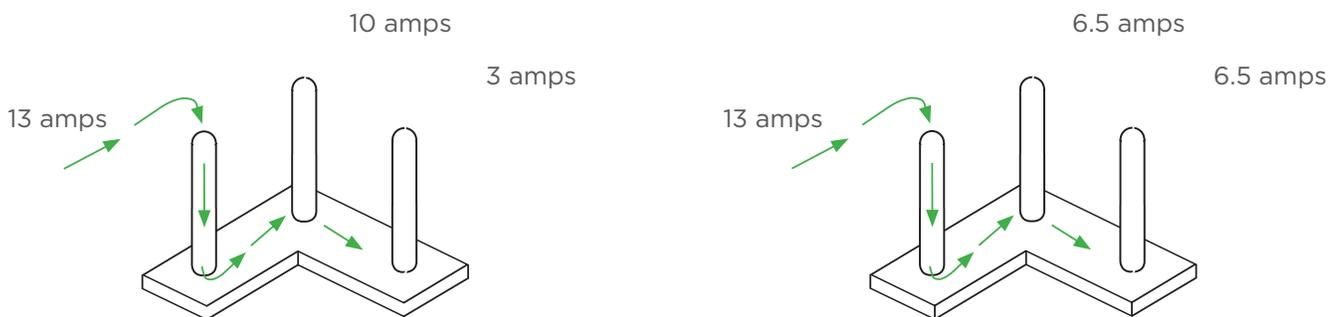
In the examples, there are three size 16 pins each rated for 13 amps mounted to the buss. A total of 13 amps can be pulled into one pin and going out the 13 amps are split between the remaining two pins. No more than 13 amps can go through any single pin.
