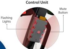
Alarm Sounder Vehicle To Vehicle Unit Communicates with other V2V units
